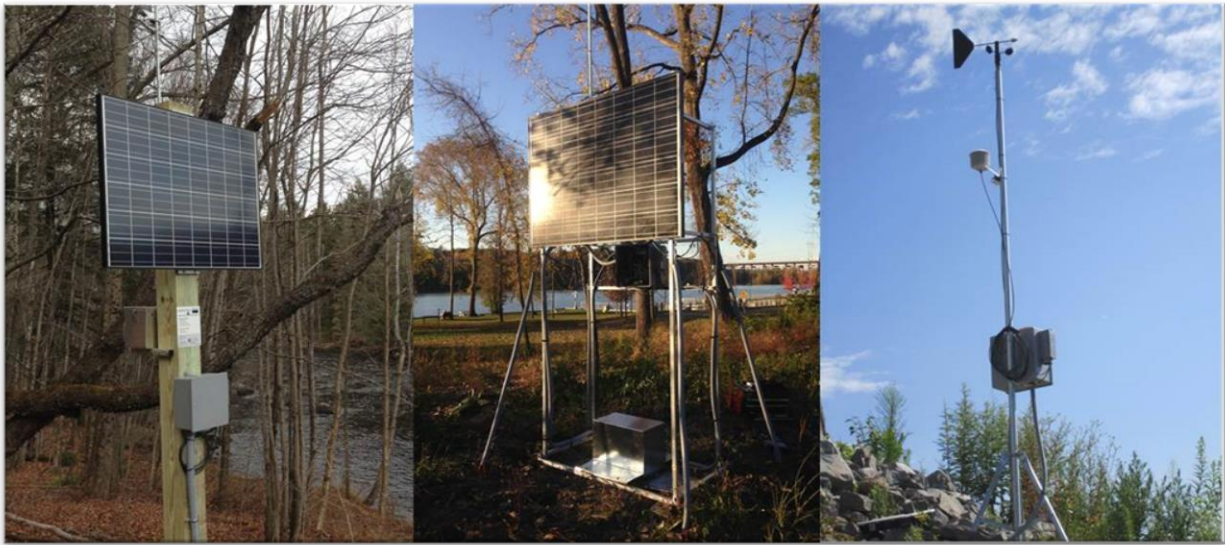
Figure 3: RTHS mounted to a timber pole (left), aluminum frame (center), and tripod (right).
