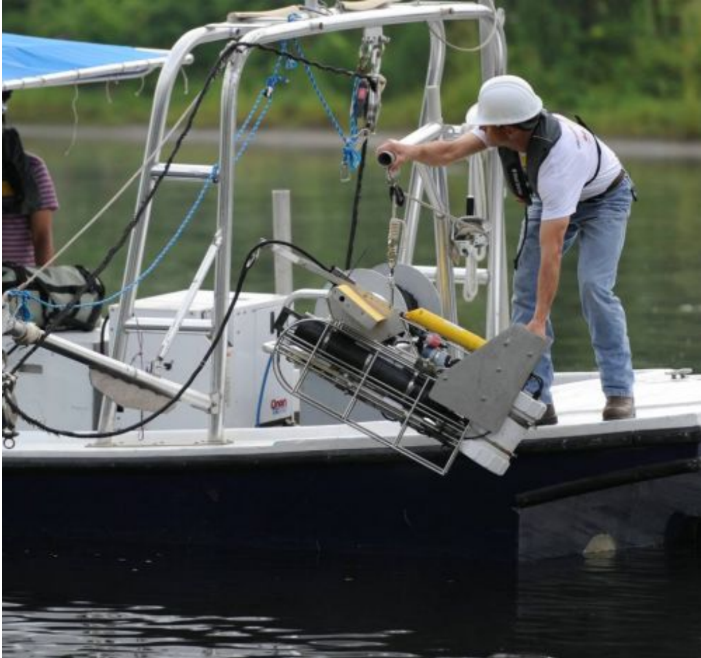
Fig. 4.2 Mobil monitoring platform. Instrument suite including particle analyzer, conductivity- temperature-depth (CTD) sensor, dissolved oxygen sensor, and fluorometer are mounted to the computer controlled undulating tow body, allowing sensor parameters to be mapped over horizontal and depth axis.
