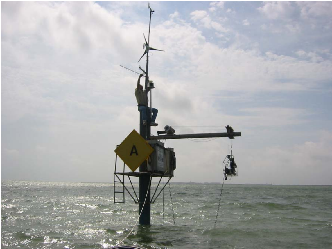
Fig. 4.3 Fixed platform in Corpus Christi Bay, WATERs test bed. Robotic profiler provides autonomous depth profiles of water quality parameters including salinity, dissolved oxygen, particle concentration and size distribution, and fluorescence.
