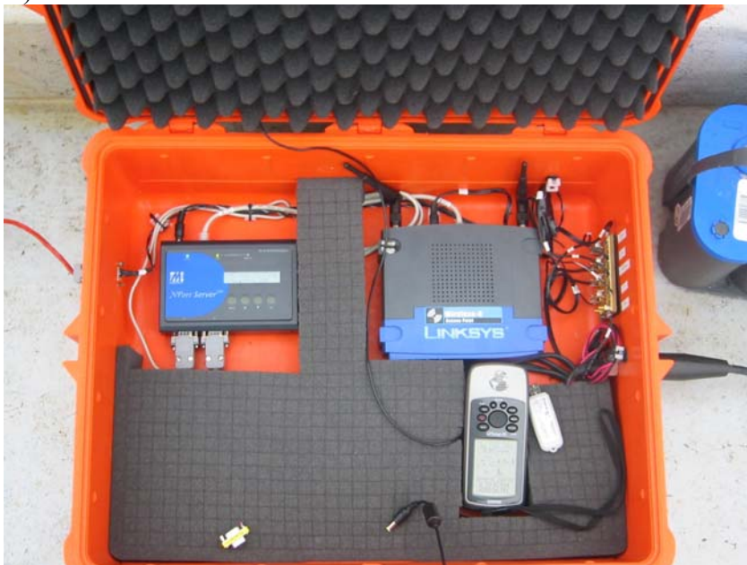
Fig. 4.1 Integrated in-situ fluorometer with GPS for tracking dispersed oil plume. A) WETLabs WETSTAR Color Dissolved Organic Material (CDOM) fluorometer mounted to lead tow-fish, B) net work interface to combine GPS and WETSTAR data streams.
