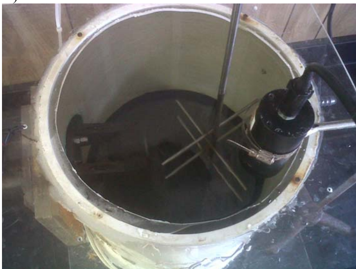
Fig. 4.4 Cylindrical 40 liter reactor vessel. A) Side view showing LISST with horizontal orientation and mixer mounted above, B) top down view showing LISST sensor head in reactor vessel with mixing impeller. Small black cylinder in ring stand is WETLabs FL3 fluorosensor.
