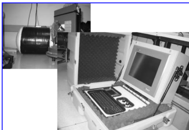
Figure 4. Submersible multi-port device server (top). IDACC comprising GPS unit, industrial computer in NEMA 4x enclosure, NEMA keyboard, power distribution, and four-port network interface. The main unit, which houses the electronics, tilts up into operating position, supported by gas springs.
