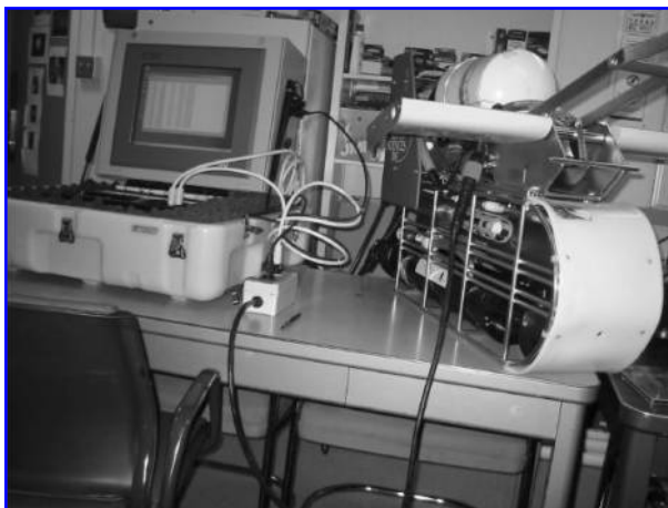
Figure 5. IDACC and tow body with instrumentation and submersible multi-port device server undergoing bench tests.
